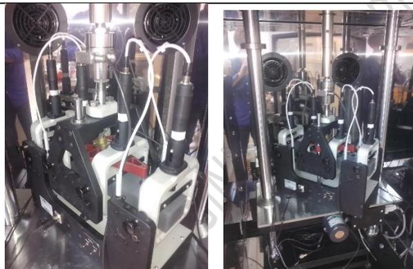
**EN 12697-26**, Bituminous mixtures — Test methods for hot mix asphalt — Part 26: Stiffness.
