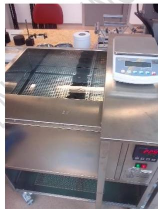
**EN 12697-8**, Bituminous mixtures — Test methods for hot mix asphalt — Part 8: Determination of void characteristics of bituminous specimens.
