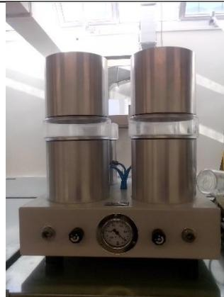
**EN 12697-6**, Bituminous mixtures — Test methods for hot mix asphalt — Part 6: Determination of bulk density of bituminous specimens
