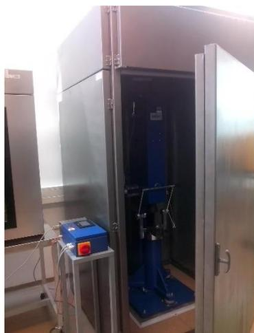
**EN 12697-31**, Bituminous mixtures — Test methods for hot mix asphalt — Part 31: Specimen preparation by gyratory compactor.
