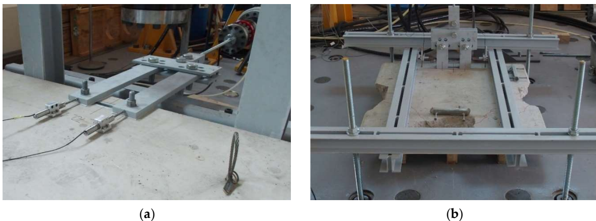
Figure 3.3 Test setups: (a) shear load; (b) tension load
