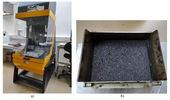
Figure 5.1 Roller compaction device (a) and produced rectangular specimen in a mold (b), Transportation laboratory Faculty of Civil engineering Rijeka, 2021
