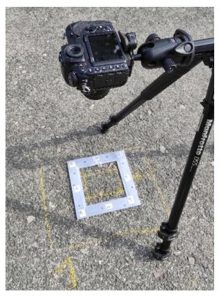
Figure 6.4 Texture data acquisition procedure by CROP methodology, 2023
