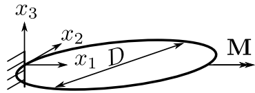
Figure 4.43: Twisting of a ring: setup
