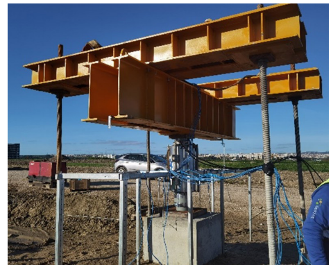
Figure 8 Reaction structure for the compression full scale load test
