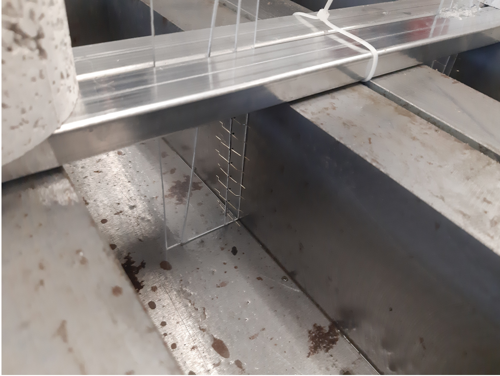
Figure 4.3: Fibers positioned in the mold before concrete pouring
