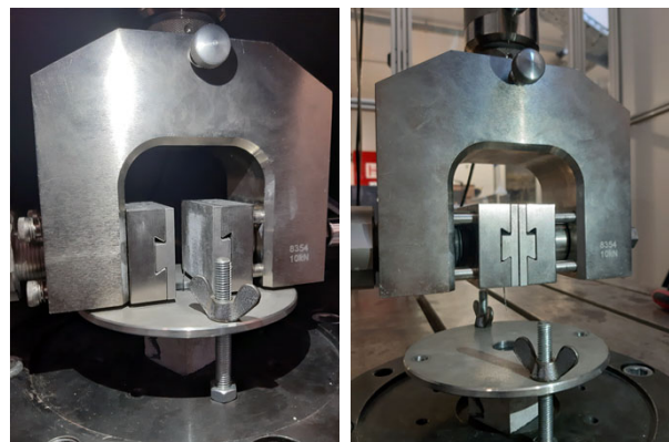
Figure 4.7: Single fiber pullout setup. Left) Prior to fiber pull-out; Right) After the fiber pull-out
